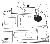
(Sample Illustration) Removing the battery
